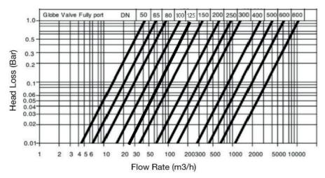
Flow curve of the main valve at fully open status
